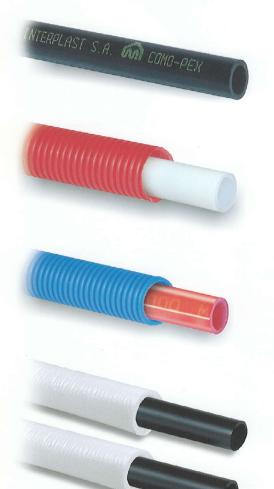
Due to their cross linked structure, **ComoPEX pipes have thermal memory** which allows them to recover in their first structure after a thermal stress. In other words, the internal structure of the material "remembers" the initial form that has been given during its production.
